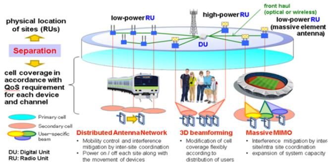
Figure-4: Virtualization of Cells
