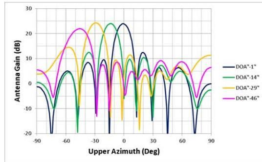
Figure-5: Measured AAS Beam Pattern
