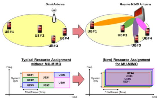
Figure-1: Intra-cell capacity enhancement on MU-MIMO with Massive-element Antenna
