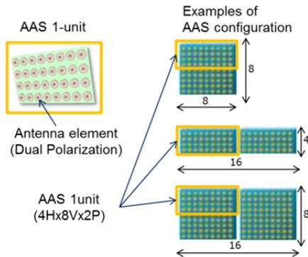
Figure-4: Examples of the AAS configuration
