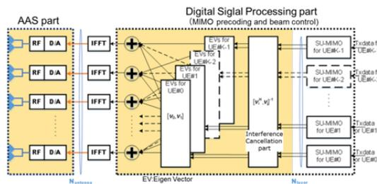
Figure-3: Block diagram of Massive MIMO
